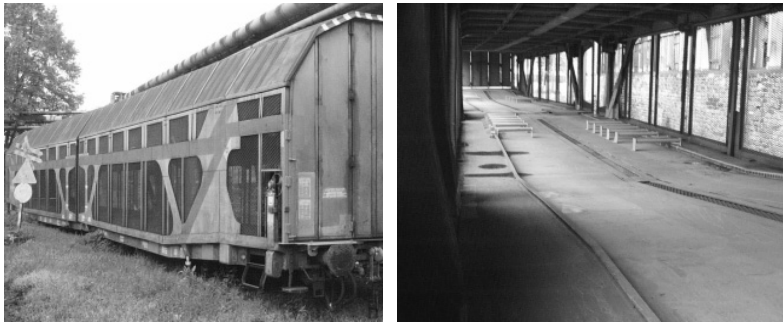
Fig. 2. Outside (left) and inside (right) view of DDam type of wagon
